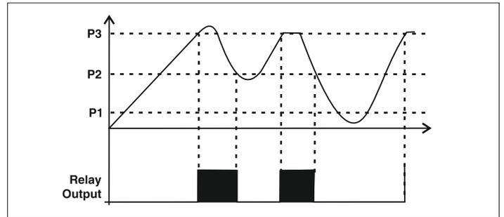
Two Level Controller for Both Tank
