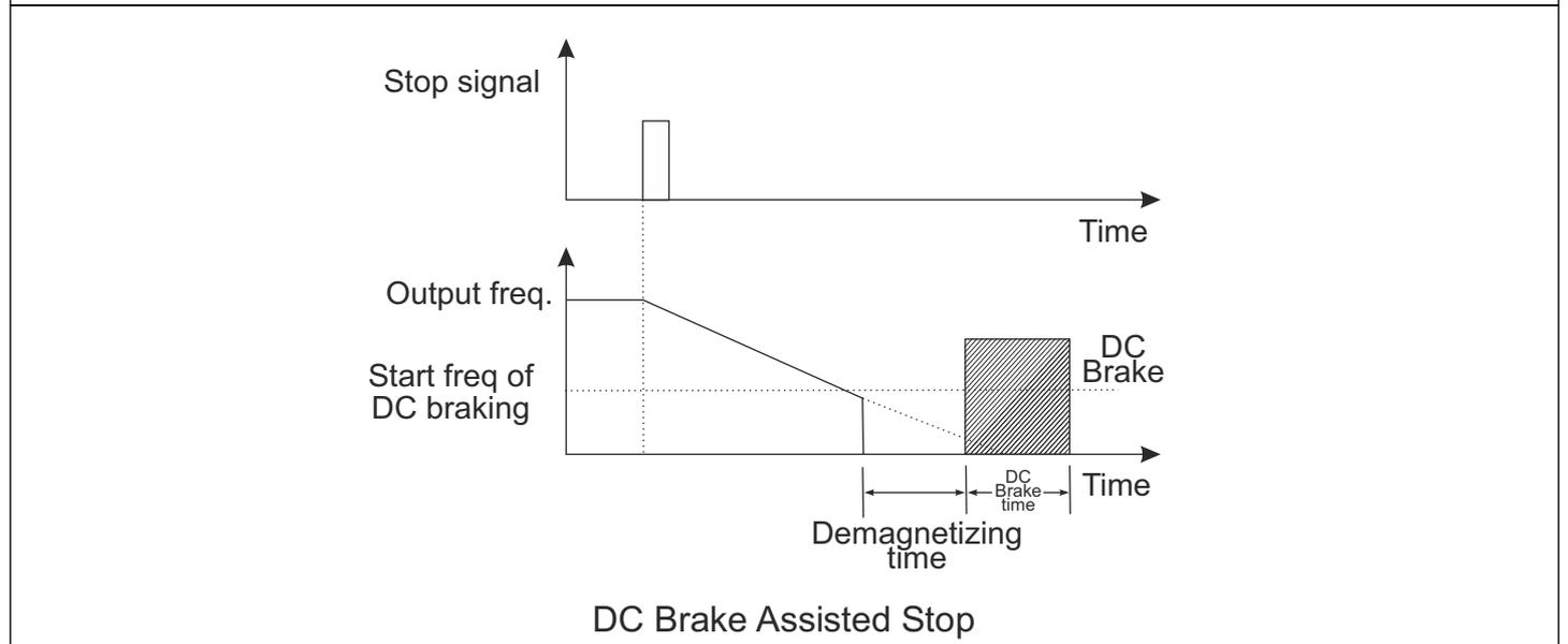
This parameter determines how the drive executes the stopping operation
