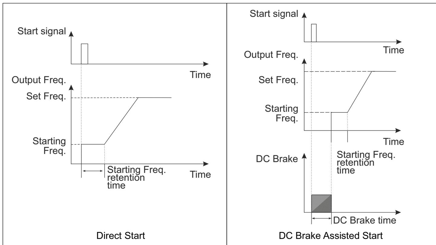
The start mode determines how the drive will initiate its operation when the RUN command is given through the selected control source.
