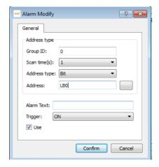
**3.** Add an alarm control, and change the corresponding display parameters.
