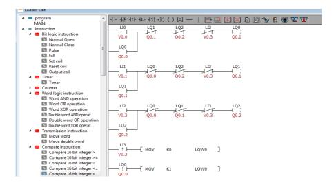
C. After editing the ladder diagram, the relevant controls can be placed in the screen, and the relevant logic is already operation.
