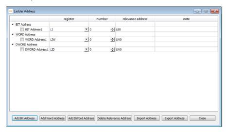
B. Ladder diagram Programming is based on ladder address. During programming, click to display the relevant address for easy writing.
