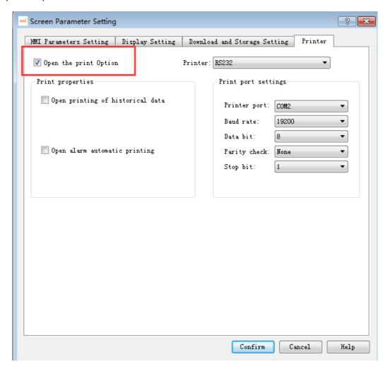
2. Choose to open the printing history data. There are two options below. One is the printing time and the other is the printing date. When neither option is checked, the printer only prints the value; when the printing time is checked, the printer prints the time plus the value; when the printing date is checked, the printer prints the date plus the value.
