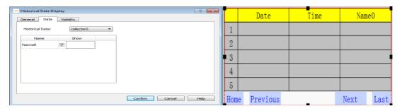
After the device operating, on HMI it will display the change of the corresponding component address variable value, and data will be saved when power off .
