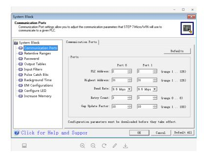
© Connect the HMI to PLC through 485 communication cable and power them together, then download the corresponding project to HMI. When click the components on the screen, the corresponding PLC output points will be lighten.
