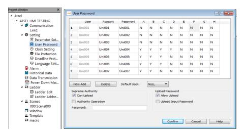
2. To encrypt a control, at "advanced" select controlled by user level, set the corresponding level, if setting level is B, then the user with the B level can use it. Display element invalid logo has an invalid touch on the current control.
