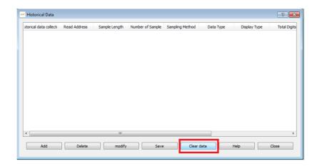
2. It controls the suspension sampling or clear historical data by address variables. Set the corresponding control address the corresponding state of the address variable is triggered the relevant function.
