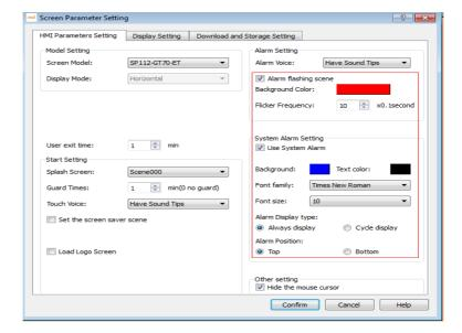
4. Clear alarm voice:the alarm sound can be set on/off by the function button
