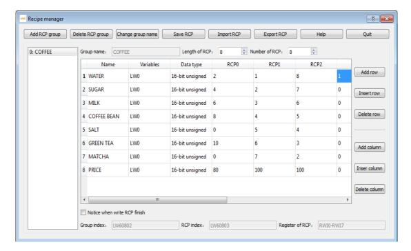
Add the corresponding components and set corresponding variables to project scene, and group index is modify Internal Register LW60802 can achieve switch-over of recipe
