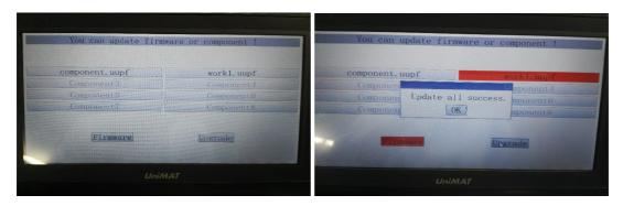
8. Pull out the U disk and restart the touch screen to complete the U disk update.
