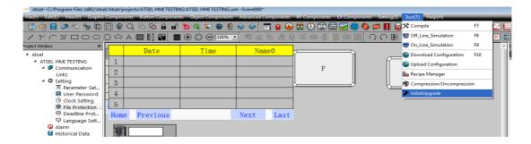
2. Pop up the U disk update window to update the configuration and firmware of the current project, and update the three files to the U disk. Mode of operation: choose the firmware and click the "..." on the right, select save path and store it in the U disk. Click confirm. Check the configuration again, click on the right "..." select save path and store it in the U disk. Click confirm.
