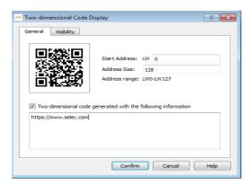
2. Two-dimensional code is controlled by address variable
