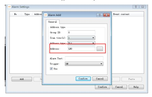
4. Set relevant trigger conditions, when the alarm event triggers, the printer will automatically start printing alarm information.
