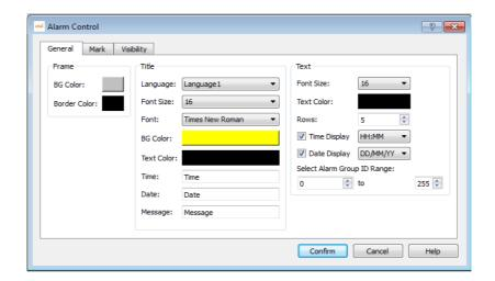
**4.** When the corresponding alarm event is triggered, the Alarm Control will display the alarm time, date and content, etc.
