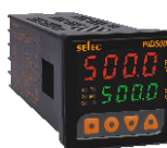
PID500-T 48(H) x 48(W) x 100(D)mm
