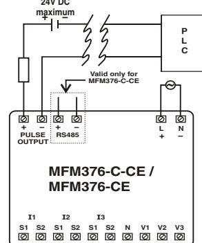
Pulse output from MFM376-C-CE / MFM376-CE meter can be interfaced into a process through a PLC for on line control of energy content in the process. If the PLC has a self excited digital input, external DC supply is not needed.
