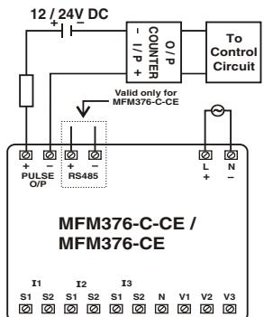
Pulse output from MFM376-C-CE / MFM376-CE meter can be used as alarm generator or total energy controller by interfacing it with Pre-settable counter and control circuits (Contactors, Relay, Trip Circuit).
