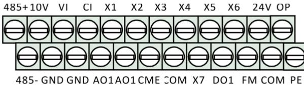
Fig. 3-6 Sequence diagram of control board terminal
