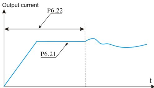
Fig.6-28 PID initial value function
