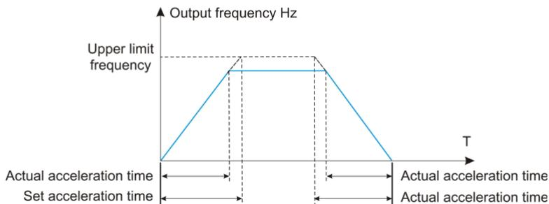
Fig. 6-1 Acceleration/Deceleration time
