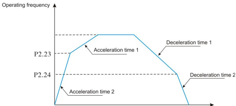
Fig. 6-12 Acceleration/deceleration switching
