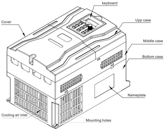
Fig 2-3 parts of Inverter
