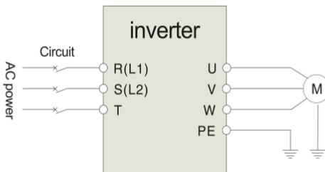
Fig. 3-3 Main circuit wiring
