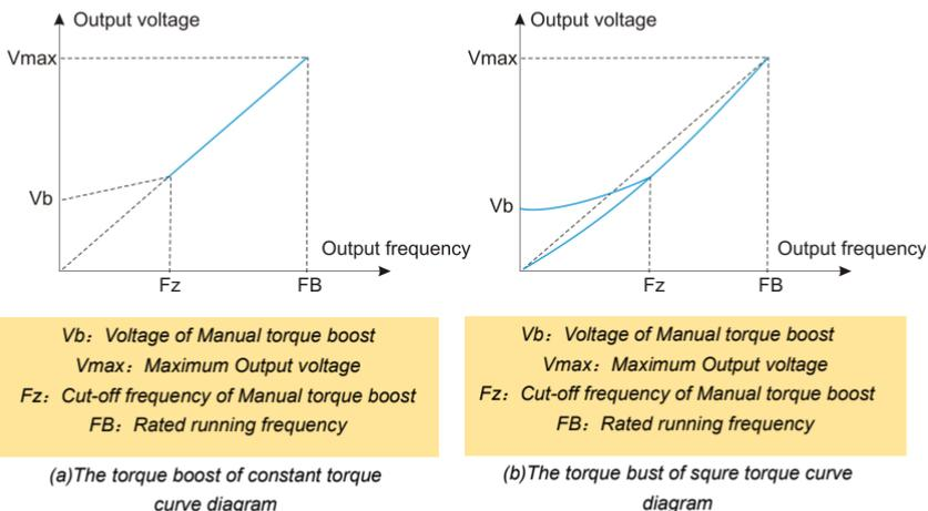
Fig.6-24 Manual torque boost
