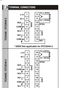
Use only the correct thermocouple wire or compensating cable from the probe to instrument terminals avoiding joints in the cable if possible. Failure to use the correct wire type will lead to inaccurate readings.
