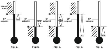
Deviation high alarm Deviation low alarm Deviation band alarm Full scale high alarm Full scale low alarm
