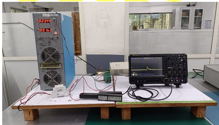
Figure 3: Inrush Current Measurement Test Setup
