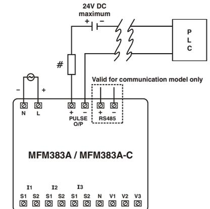
Pulse output from MFM383A meter can be interfaced into a process through a PLC for on line control of energy content in the process. If the PLC has a self excited digital input, external DC supply is not needed. The kWh pulse is also used to derive average kWh information at the PLC.
