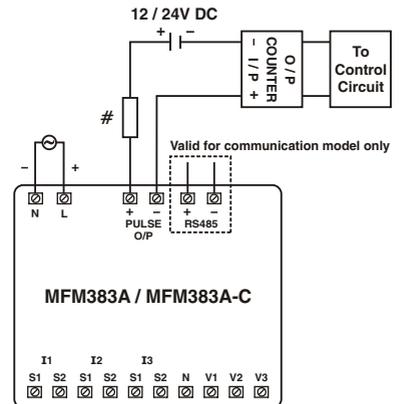
Pulse output from MFM383A meter can be used as alarm generator or total energy controller by interfacing it with Pre-settable counter and control circuits (Contactors, Relay, Trip Circuit).
