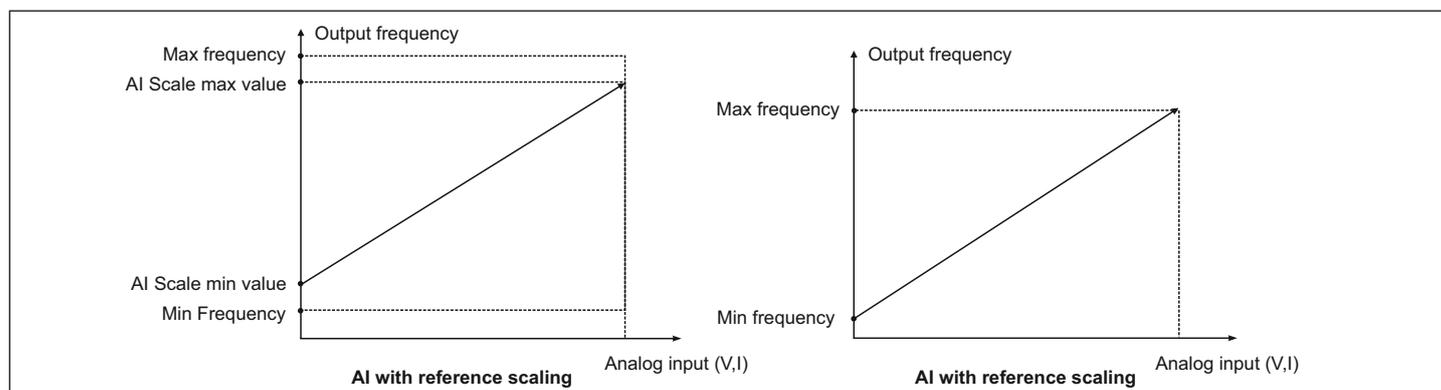
Fig.6.10 AI With and Without Scaling
