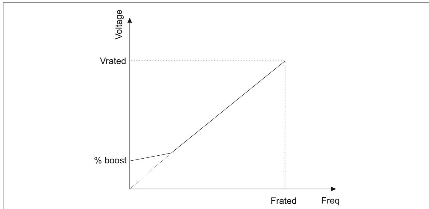
Fig.6.9 Torque Boost
