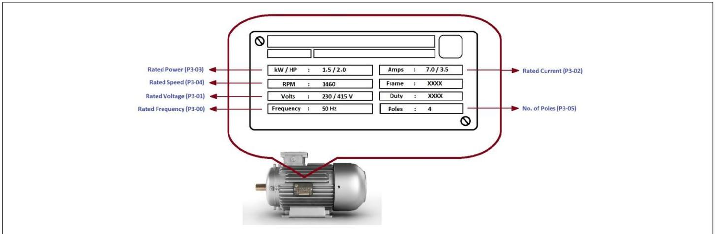
Fig.6.6 Motor Parameters
