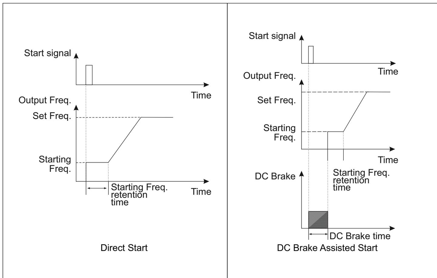
Fig.6.2 Direct Start and DC Brake Assisted Start
