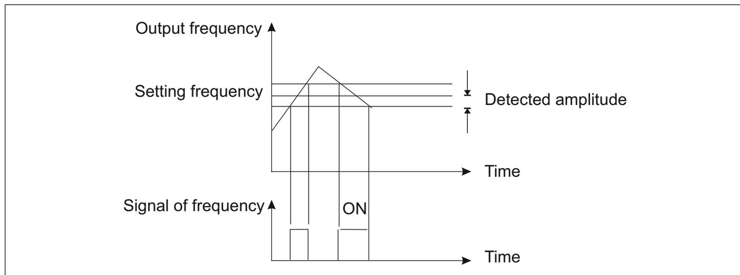
Fig.6.16 Amplitude of Frequency Arrival
