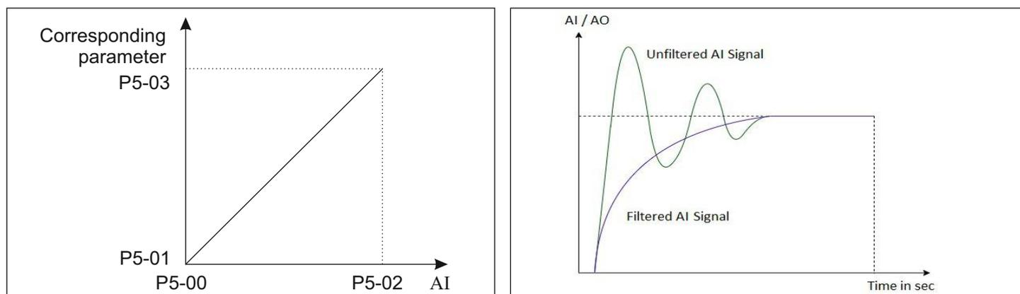
Fig.6.11 AI With and Without Filtering
