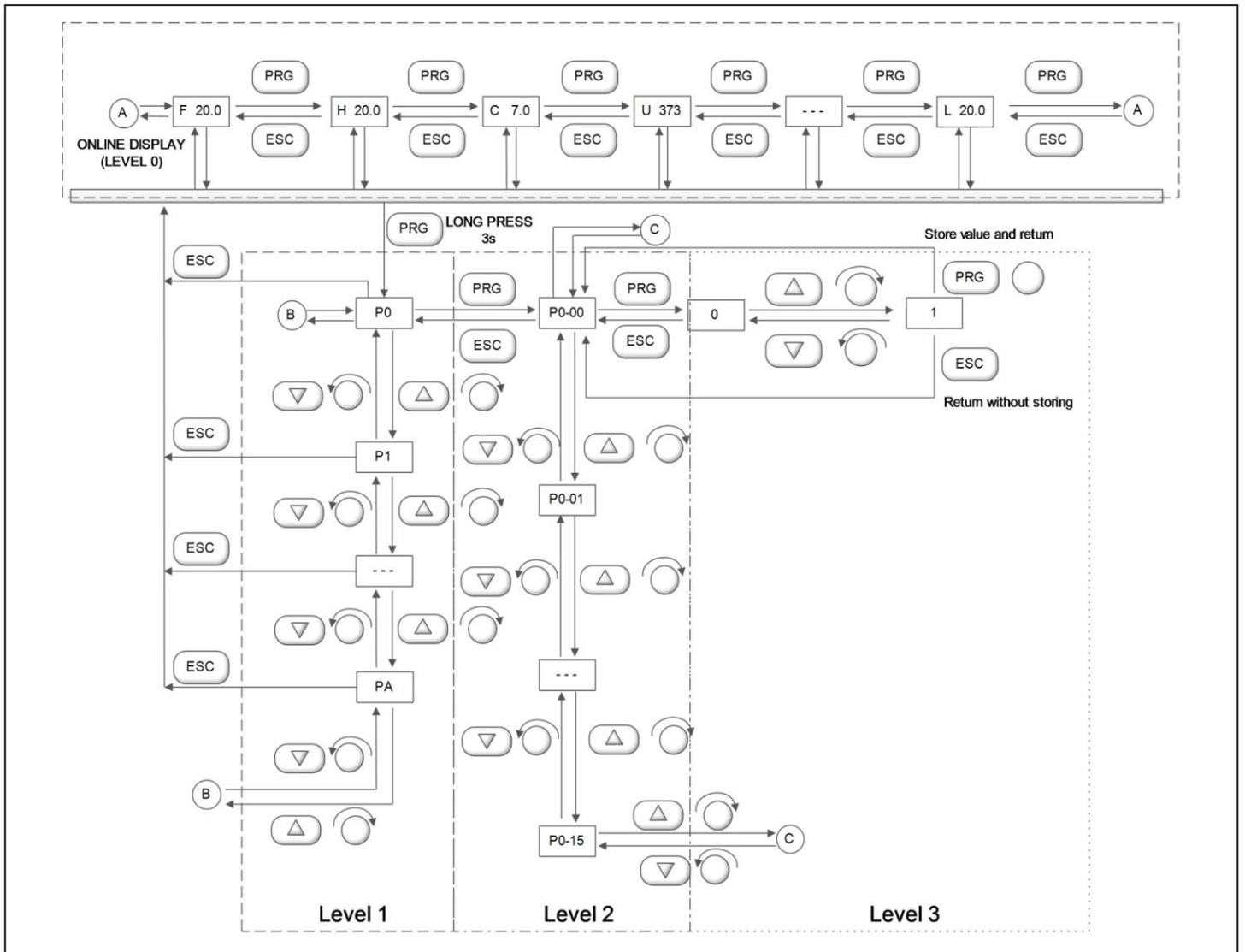
Fig.4.2 Illustration of Keyboard Operations
