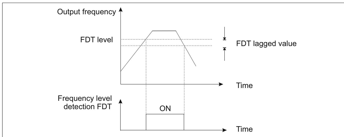
Fig.6.15 Frequency Detection Level
