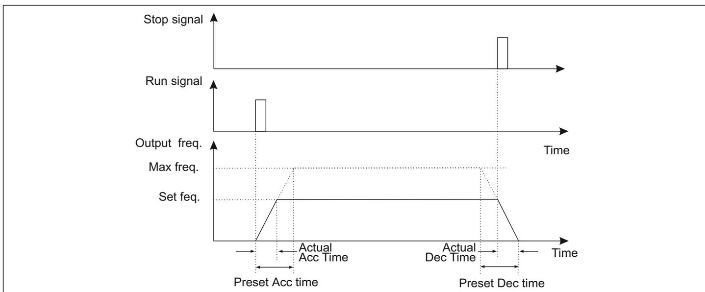
Fig.6.1 Acceleration and Deceleration
