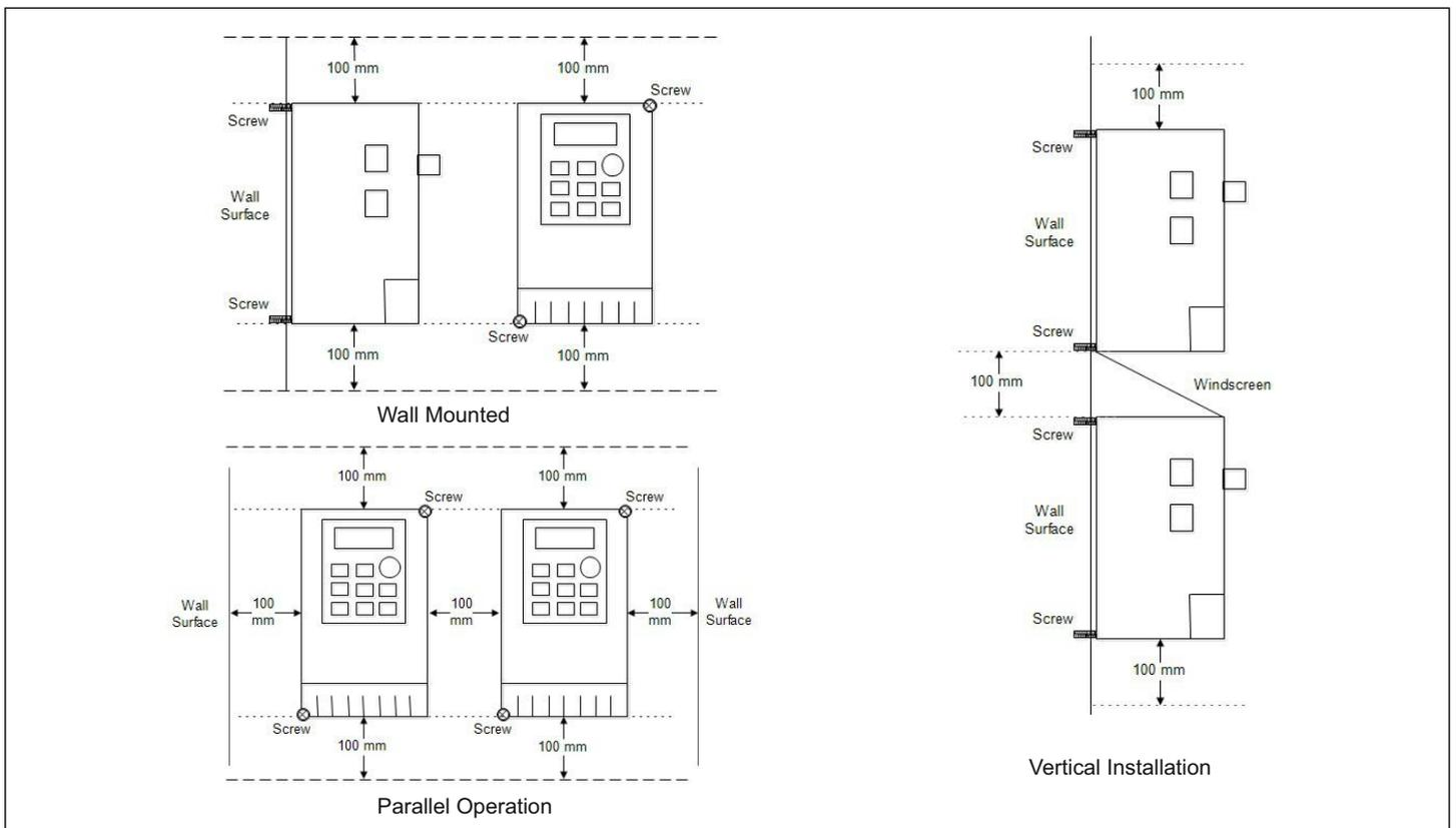
Fig.2.1 Separation While Installation
