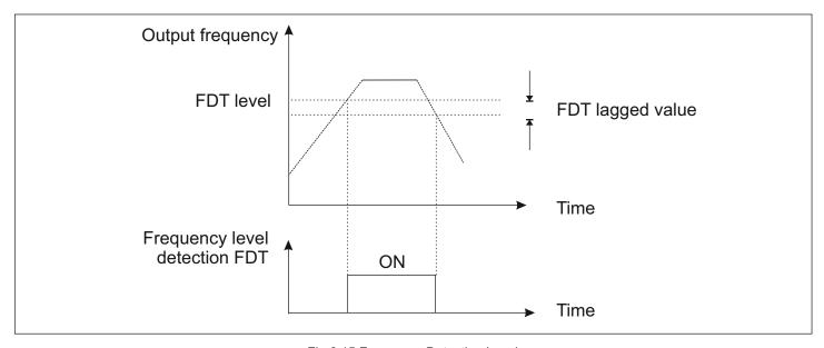
Fig.6.15 Frequency Detection Level
