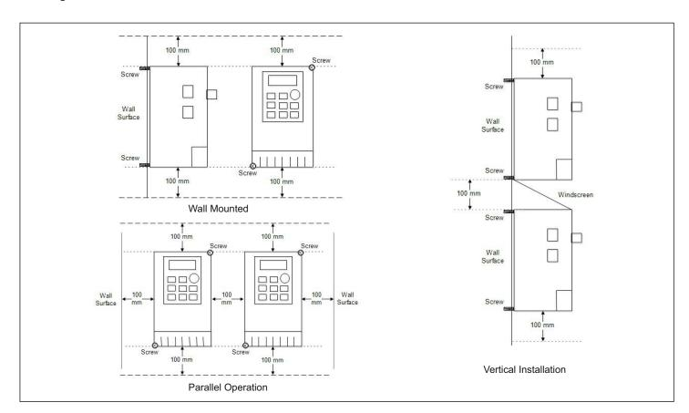
Fig.2.1 Separation While Installation
