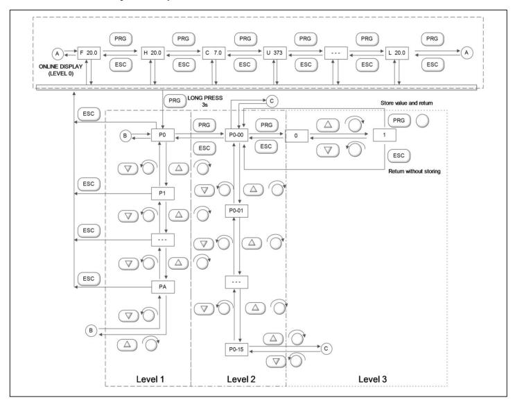
Fig.4.2 Illustration of Keyboard Operations
