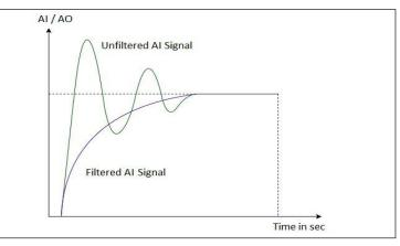
Fig.6.11 AI With and Without Filtering
