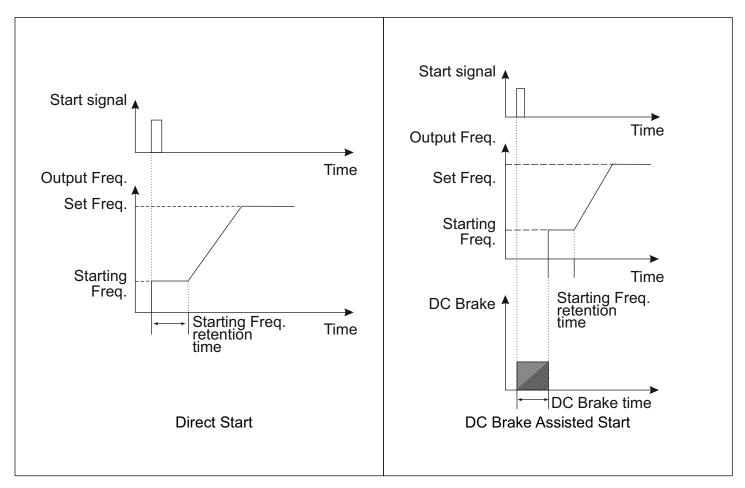
Fig.6.2 Direct Start and DC Brake Assisted Start
