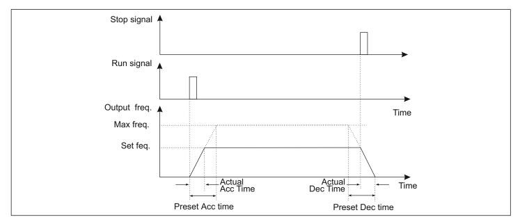
Fig.6.1 Acceleration and Deceleration
