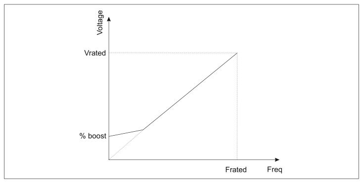
Fig.6.9 Torque Boost
