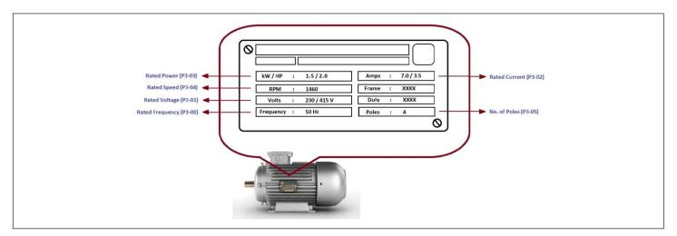
Fig.6.6 Motor Parameters
