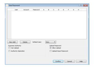
Note: when a user has multiple levels of authority (for example, A/B/D), as long as it is unlocked in one of the controls, the corresponding all permissions are unlocked (when the A is opened, B and D are open at the same time, before logon the login, no more password is required).
