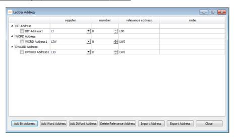
Ladder diagram Programming is based on ladder address. During programming, click to display the relevant address for easy writing.
