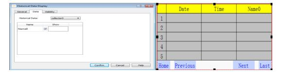
After the device operating, on HMI it will display the change of the corresponding component address variable value, and data will be saved when power off .
