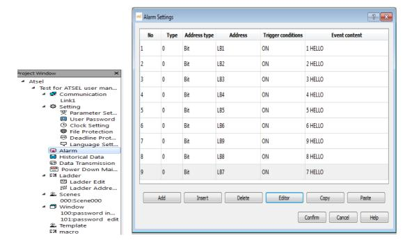
2. Add the matched alarm event in the alarm setting and change the trigger condition.
