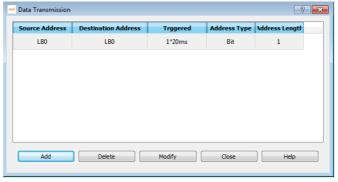
3.After adding, click close button exit, after downloading the configuration you can do data exchange according to the set transmission type.
