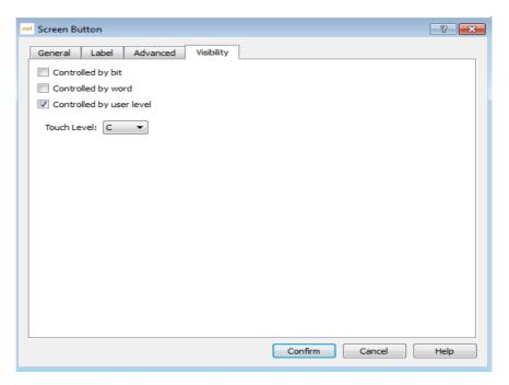
The Supreme Authority Operation is that the task user enters the corresponding password and then can operate on all controls.
