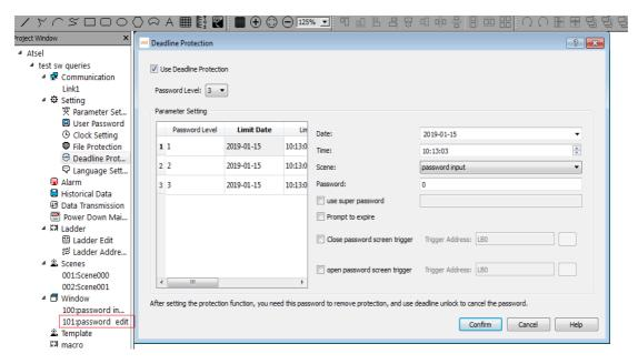
B.Click on the password input window, set the corresponding manufacturer and contact information, and put the corresponding payment two-dimensional code. The image of this window screen can be user-defined edited.
