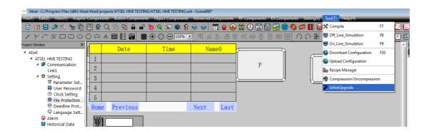
2. Pop up the U disk update window to update the configuration and firmware of the current project, and update the three files to the U disk. Mode of operation: choose the firmware and click the "..." on the right, select save path and store it in the U disk. Click confirm. Check the configuration again, click on the right "..." select save path and store it in the U disk. Click confirm.
