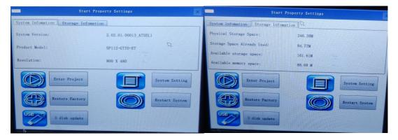
System settings, in the system settings, you can view the current system information, including the current application software version number, version type, and the IP address of the machine (if no Ethernet shows no support); can adjust the backlight brightness through a scroll bar; in calibration, the touch screen can be calibrated; IP The address can set the IP of the Ethernet HMI.
