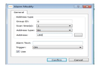
3. Add an alarm control, and change the corresponding display parameters.
