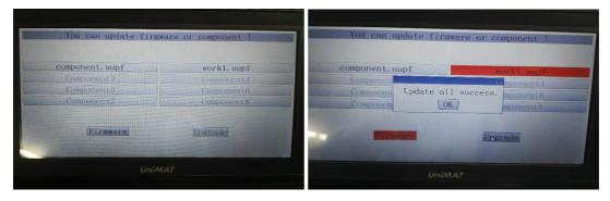
7. Pull out the U disk and restart the touch screen to complete the U disk update.
