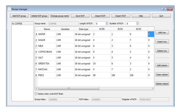
Add the corresponding components and set corresponding variables to project scene, and group index is modify Internal Register LW60802 can achieve switch-over of recipe group, If recipe index is Modify Internal Register LW60803 can achieve recipe switch-over of recipe group.
