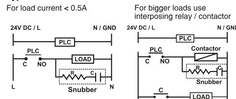
**NOTE :** A) Use snubber as shown above to increase life of internal relay.
