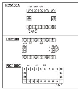
Sensor color codes and Connections:-Red = +12V. Green = CNT. Black = GND:
