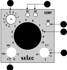
1. Red LED indicates Relay R1 & Green LED indicates Relay R2
