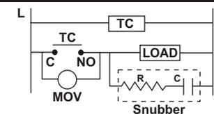
**For bigger loads, use interposing relay / contactor**
